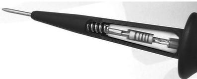
The instrument provides a high level of safety by means of two series resistors immediately behind the test electrodes as well as two absolutely independently working test systems.
