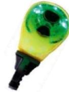
The green LED steady and **RANGE** LED, at the end of the self-test, means a low battery level requiring a future replacement.
