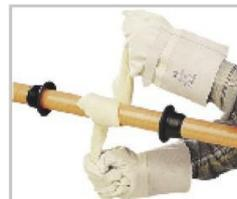
Use of silicone cloth: apply in a circular movement to be sure to break the film of damp
